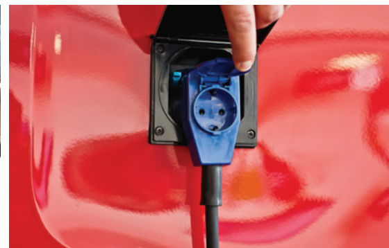
External CEE socket (for SHORT on the left, for LONG on the right) With the possibility to bring out a 230V socket under the awning
