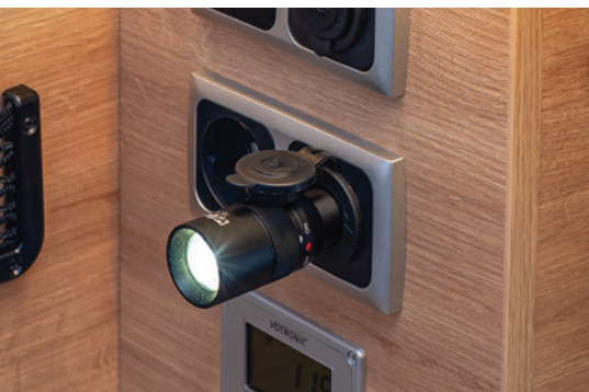
A handy flashlight charged from a 12V socket mounted in an easily accessible holder
