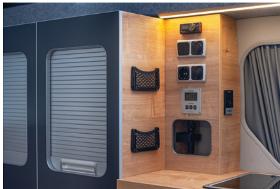
panel with double USB, 12V, 230V sockets
