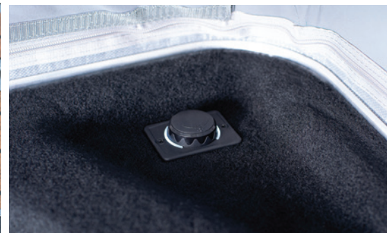
Double USB socket in the sleeping roof space
